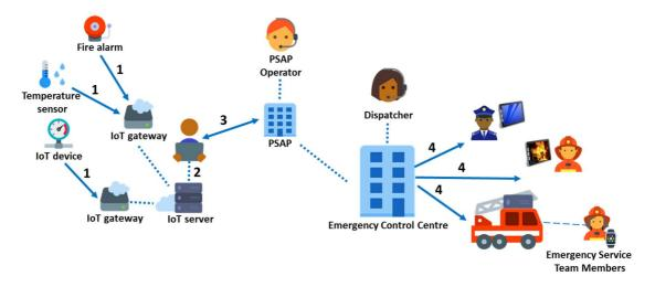
Figure 5.2.1.9-1: Illustration of automatic emergency call from IoT device
