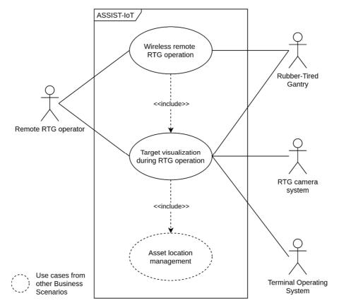
Figure 5.6.4.9-1: Illustration of RTG remote control with Augmented Reality (AR) support
