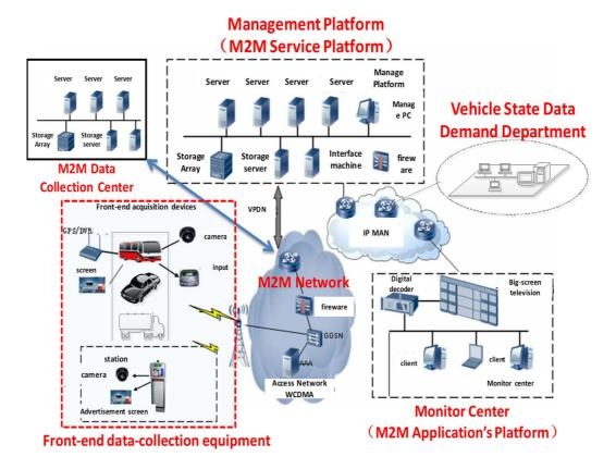
Figure 5.4.4.9-1: Vehicle Operation Management System
